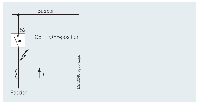
Fig. 10/8 End-fault between circuit-breaker and current transformer
