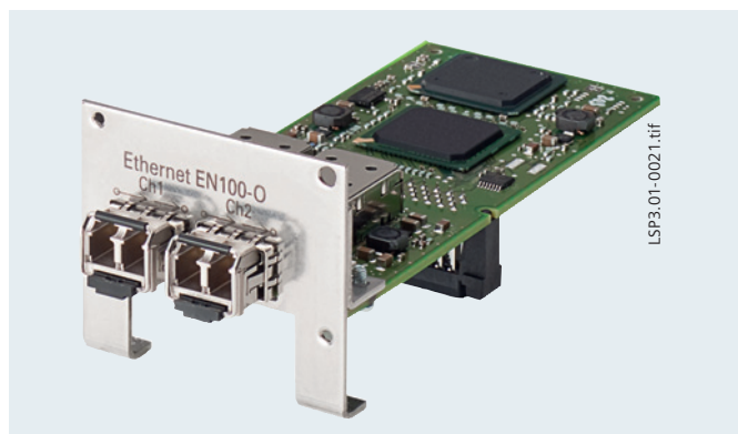
Fig. 8/17 Optical Ethernet communication module for IEC 61850 with integrated Ethernet switch
